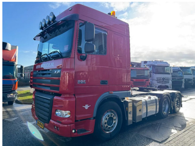
DAF XF 105.460 6X2 - EURO 5 + LIFT/STEERING AXLE
