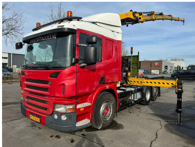
Scania P380 6X2 HIAB 288 + REMOTE CONTROL + PLATEAU
