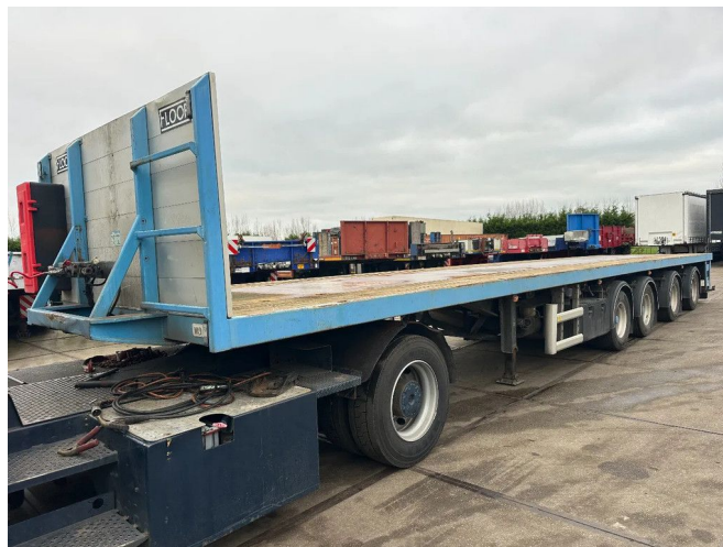
Floor 2 AXLE STEERING an 2 LIFT AXLE
