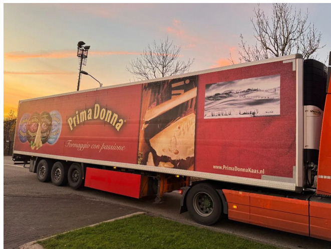
Krone SD + CARRIER VECTOR 1850 + 3X SAF AXLES
