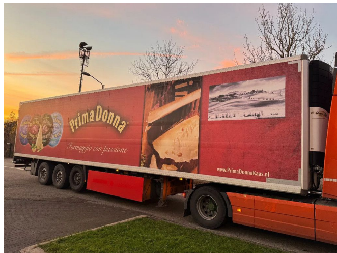
Krone SD + CARRIER VECTOR 1850 + 3X SAF AXLES
