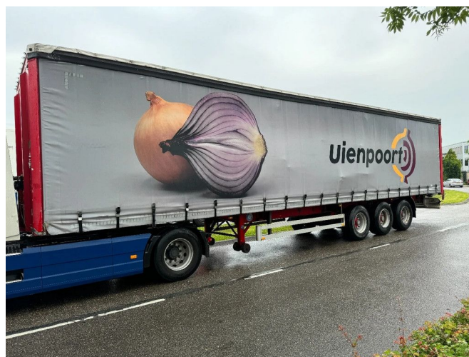
Pacton T3-001 / 3X SAF AXLE DRUM BRAKES
