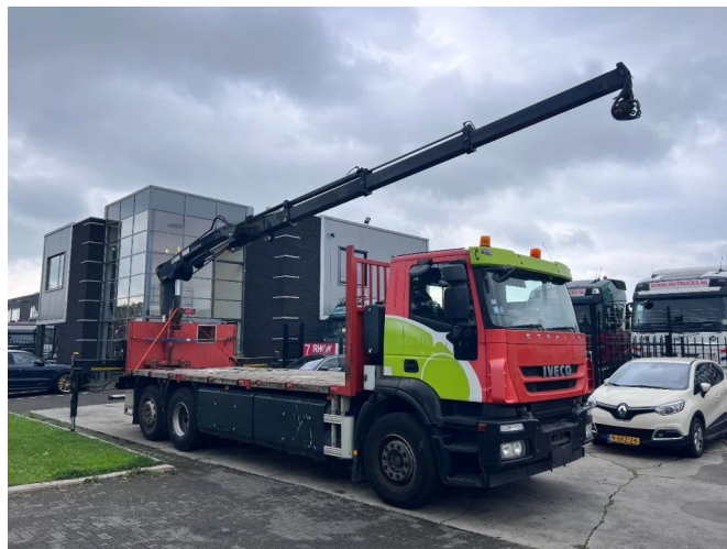
Iveco Stralis 330 CNG 6X2 INTARDER + HIAB 166 + REMOTE
