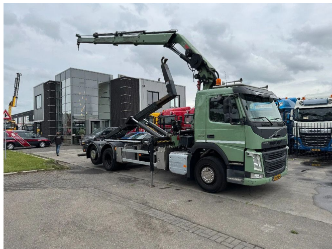
Volvo FM 370 6X2 VDL 21T HOOK + HIAB 211 + REMOTE ...
