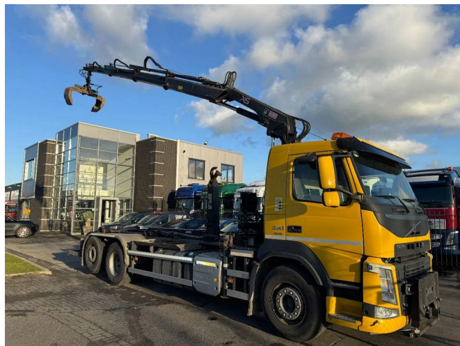
Volvo FM 370 6X2 - EURO 6 + HIAB 122 D-3 + HIAB MULTILIFT XR18S HOOK
