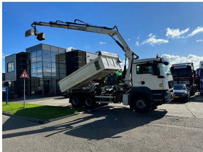
MAN TGS 26.400 6X4 HIAB 166D + REMOTE CONTROL + 2...
