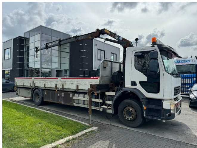
Volvo FE 280 4X2 + HMF 760 K3+2 + REMOTE CONTROL
