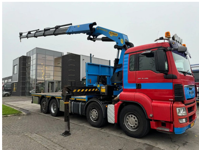
MAN TGS 35.400 8X2 + PK50002-EH PALFINGER + REMO...
