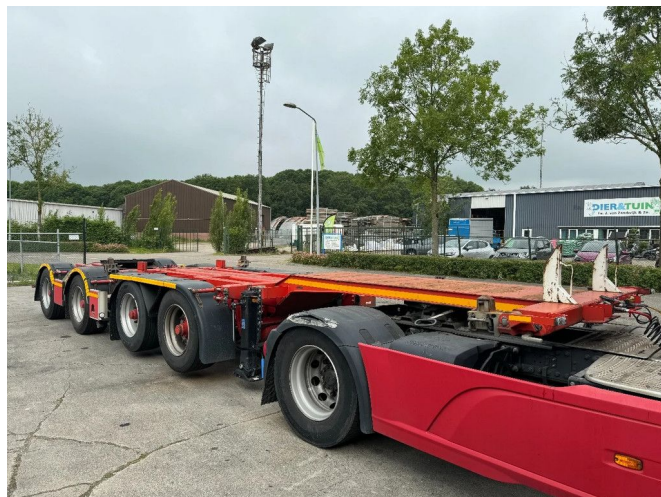
DTE CTD 44 04 - 2X STEERING 2X LIFT AXLE
