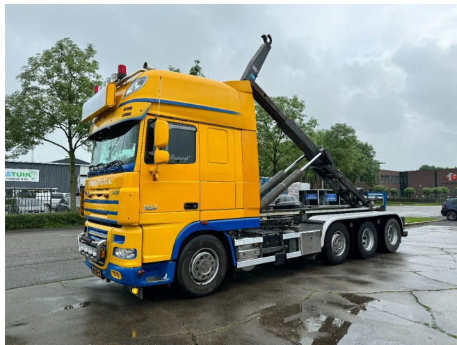
DAF XF 105.460 8X2 EURO 5 HOOKLIFT VDL 30-6500
