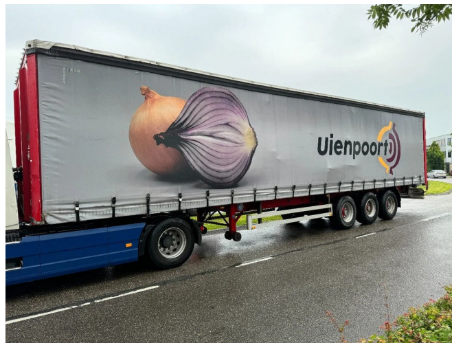
Pacton T3-001 / 3X SAF AXLE DRUM BRAKES
