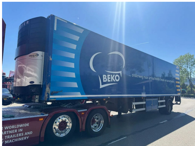
HRD SKFG - BPW AXLE + CARRIER VECTOR 1850MT
