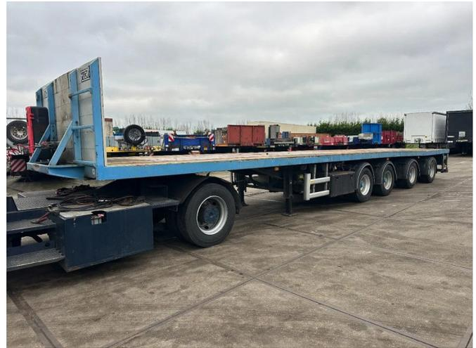
Floor 2 AXLE STEERING an 2 LIFT AXLE
