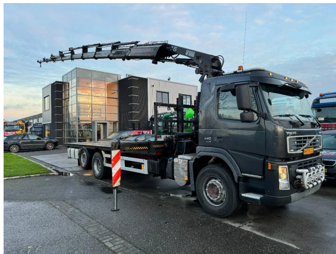
Volvo FM 440 6X2 HIAB 288E-8 + REMOTE CONTROL
