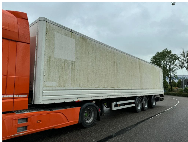
Van Hool 3B2014 3X BPW AXLE LAST AXLE STEERING
