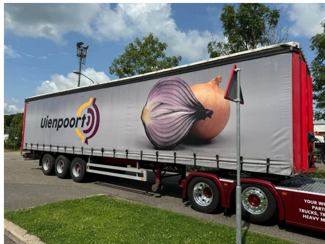
Pacton T3-001 / 3X SAF AXLE DRUM BRAKES
