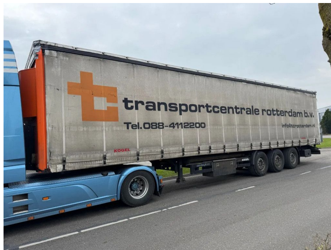
Kögel S24 - 3 AXLE SAF + SLIDING ROOF
