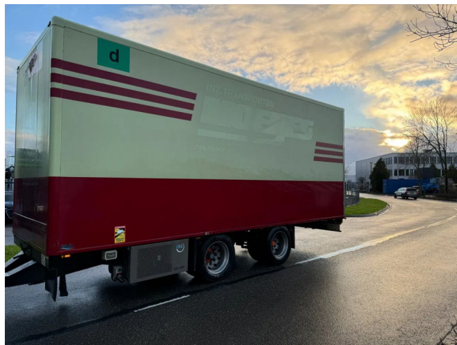
Fliegl TPS 180 - 2 AXLE BPW + TRS COOLING
