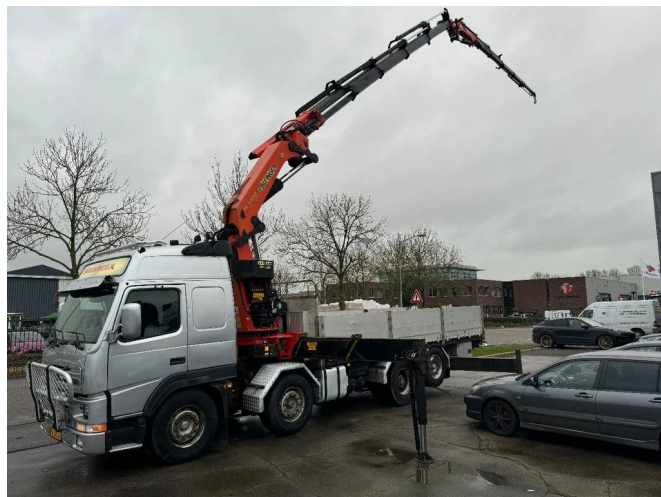
Volvo FM 12.420 8X2 PALFINGER PK44002 + JIB PJ115 + ...
